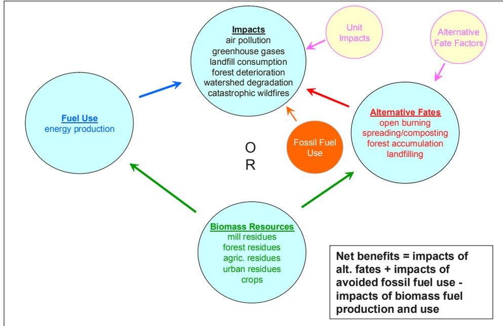
**Figure 6: Harvested Fuel Module**
